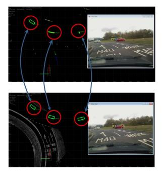
The top image shows the online results, which are improved in the offline stage using Evaluation Suite. The bottom image shows that all the labeled objects have the correct classification results, and their bounding boxes are consistent with the correct underlying class. Moreover, a map of lane markings has been built, and the labeled objects are now provided in combination with this map as the final output.
